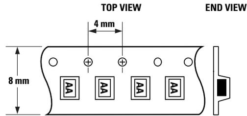
Note: "AA" represents package marking code. Package marking is right side up with carrier tape perforations at top. Conforms to Electronic Industries RS-481, "Taping of Surface Mounted Components for Automated Placement." Standard quantity is 3,000 devices per reel.
