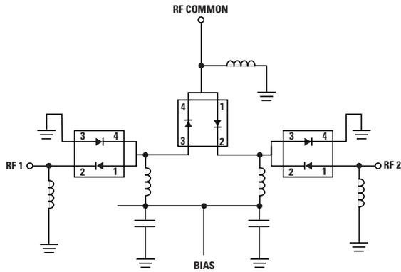
Figure 8. Very High Isolation SPDT Switch, Dual Bias.
