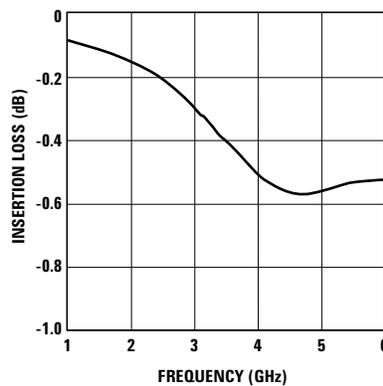
Figure 18. Insertion loss of HMPP-389T at 0V.
