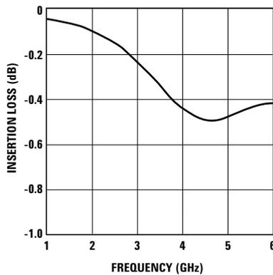
Figure 19. Insertion loss of HMPP-389T at -20V.
